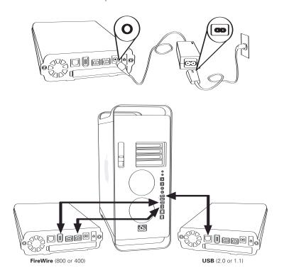
\* Only one interface port (FireWire 800, FireWire 400, or USB) can be used to connect the Maxtor OneTouch drive to your computer.
