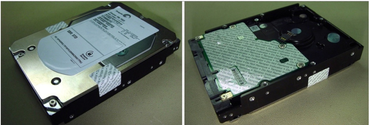
Figure 10. Example of FIPS tamper evidence labels.
