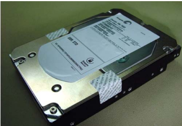
Figure 14. Example of FIPS tamper evidence labels.
