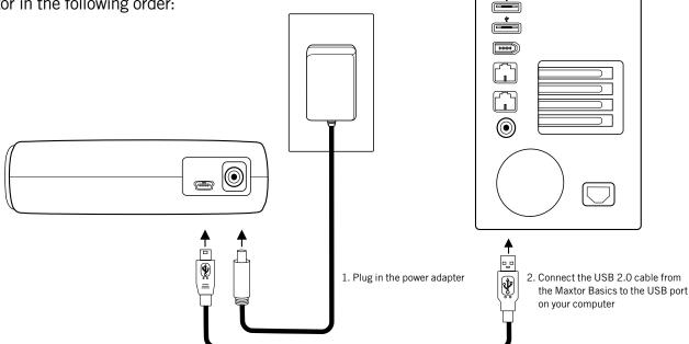
**EN** Plug in the power adapter. Connect the USB cable from the Maxtor Basics External Hard Drive to your computer.
