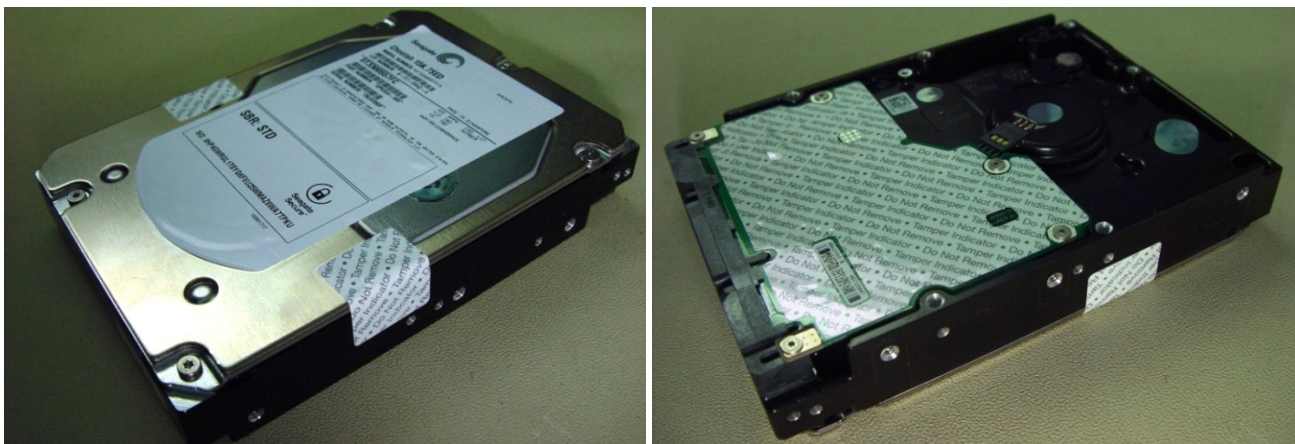
Figure 11. Example of FIPS tamper evidence labels.
