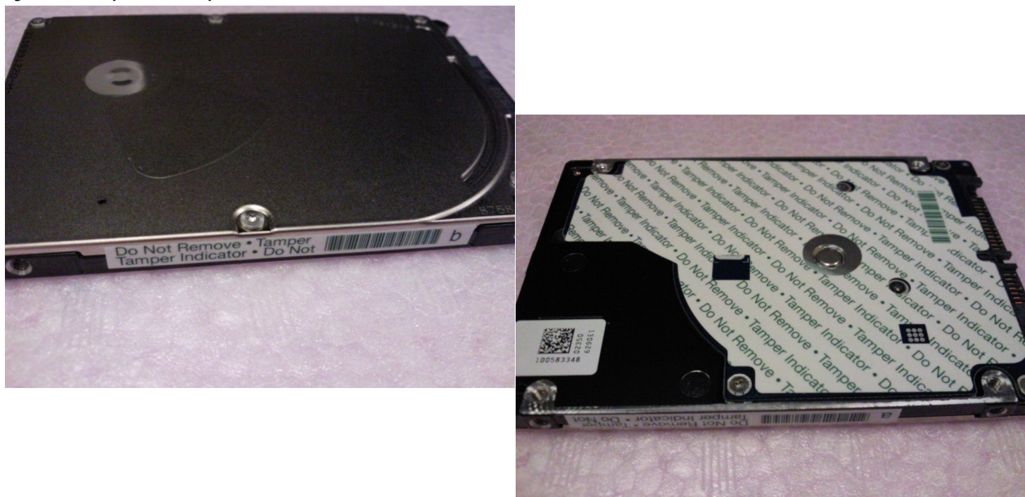
Figure 5 Example of FIPS tamper evidence labels.
