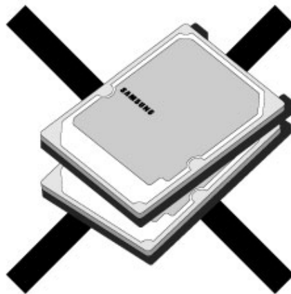
Fig. 7-2: HDD handling guide -Do not Touch Cover and PCB!
