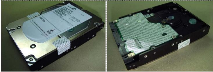
Figure 5. Example of FIPS tamper evidence labels.
