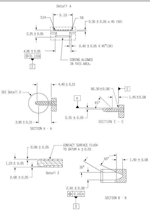
Figure 10. SAS device plug dimensions (detail)
