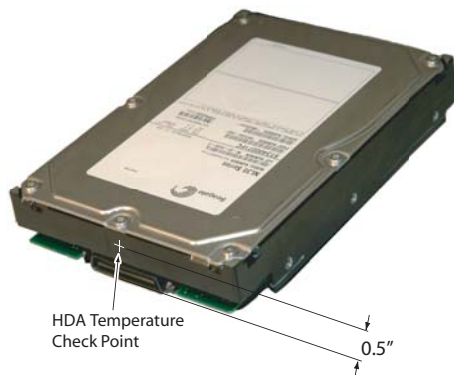
Figure 4. Location of the HDA Temperature check point
