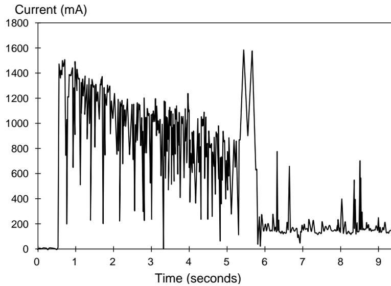
**Figure 1. Typical startup and operation current profile for the ST34340A and ST33230A**
