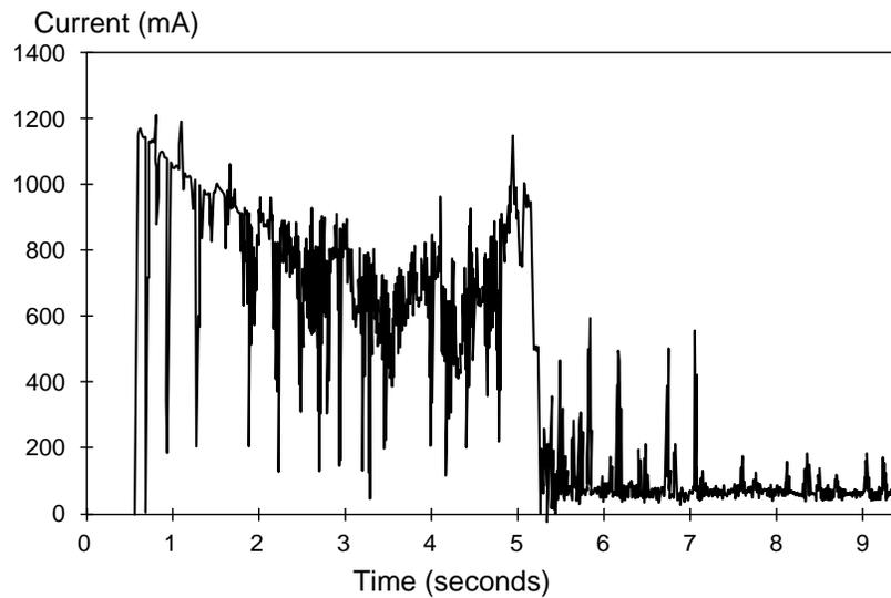
**Figure 2. Typical startup and operation current profile for the ST32120A, ST31721A and ST31010A**
