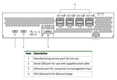
Figure 1 Ports on sample controller module
