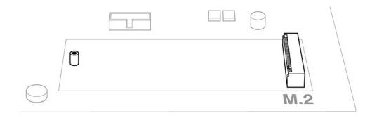
**Note** — Some motherboards have a pad installed in the **M.2\_PAD** space by default. This pad can be removed to ensure a better fit for the SSD.
