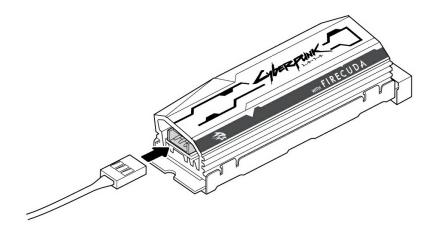
2. Connect the other end of the cable to the 5V addressable header on the motherboard. The power pin (marked with a triangle and identified by the red cable) must be connected to the 5V pin 1. Refer to your motherboard documentation for detailed instructions on how to connect RGB capable components to your motherboard. Incorrect connection can damage the RGB connector on the heatsink as well as the computer's LED function.
