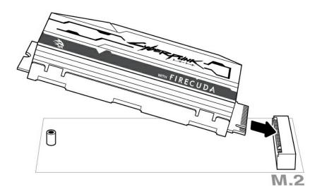
8. Hold down FireCuda SSD while you fasten the mounting screw. Make sure the SSD is secured in place.
