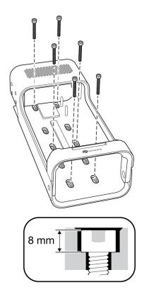
To avoid damaging Lyve Mobile Array's enclosure, the cylindrical socket cap on the mounting screws cannot exceed 8 mm in height.
