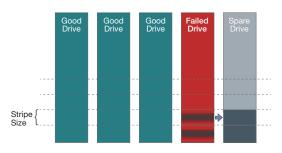
Third stripe encounters error from failed drive so data is recovered using good drives.
